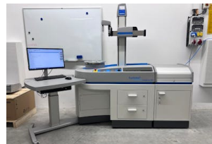
Measuring machine Hommel-Etamic, Roundscan 555 Year of manuf.: 2017, Control: Turbo Form
